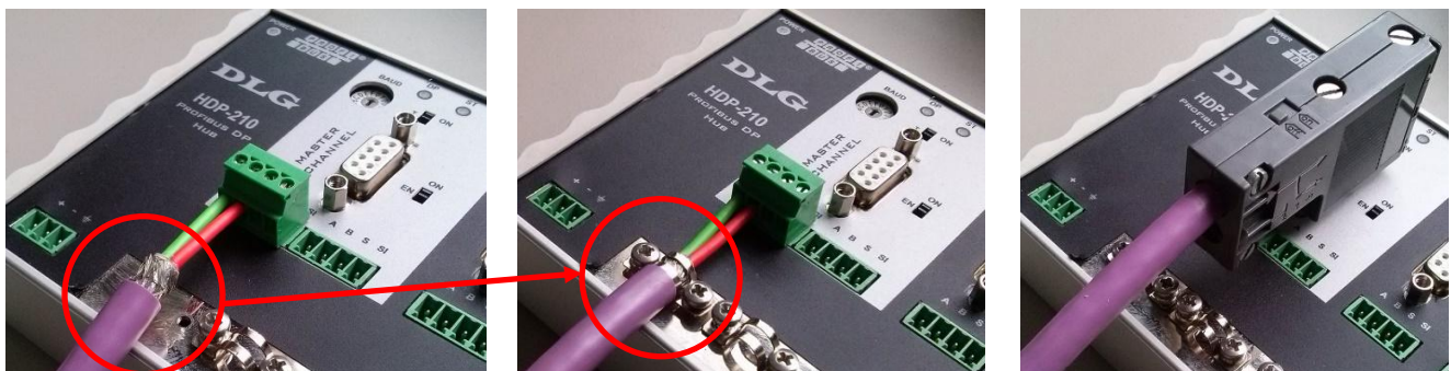
Connect the cable's shielding on the bracket
