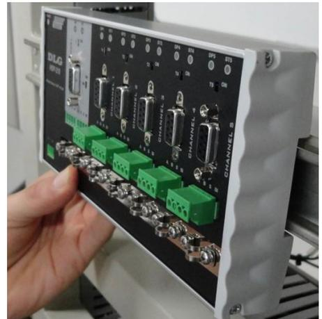
To release the HDP-210 from the rail, just push it to the bottom and next to up and pull the top out.
