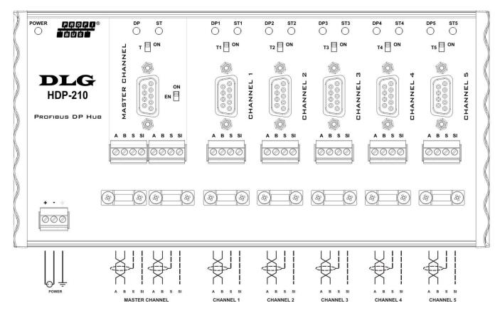
Figure 3 - HDP-210 Electric connections.
