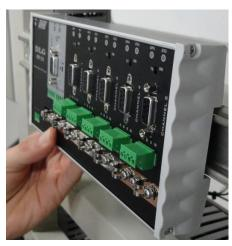
To release the HDP-210 from the rail, just push it to the botton and next to up and pull the top out.
