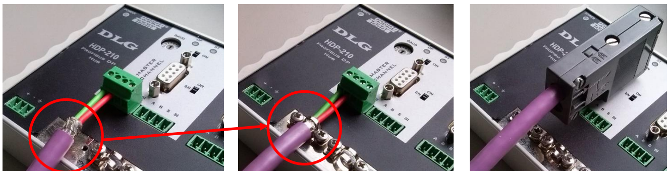
Connect the cable's shielding on the bracket
