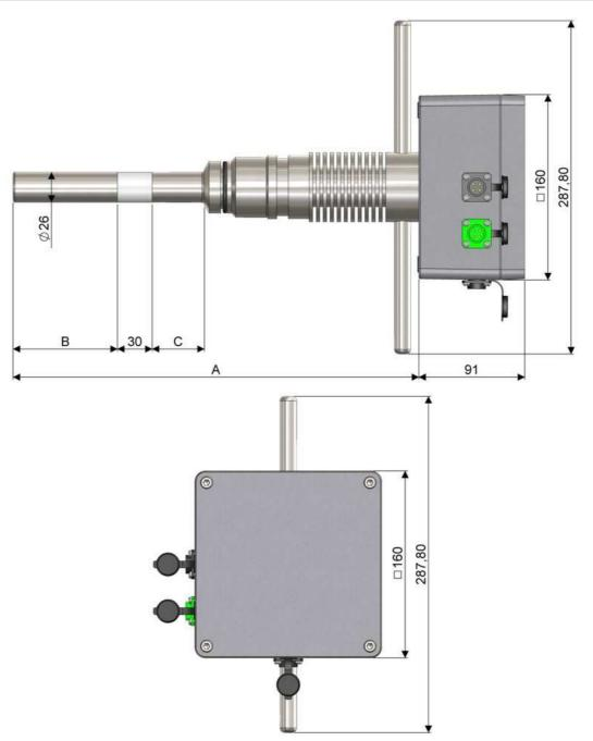
Figure 1 – Scaling mount (dimensions in mm)
