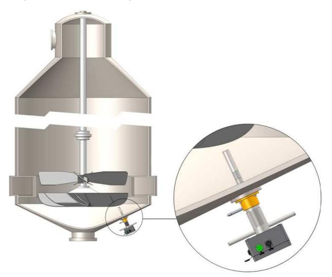
\*Figure 3 - Transmitter position in sugar cooking pot (vaccum)
