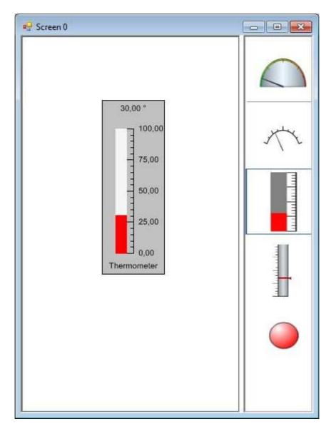
This feature allows animating all analog registers from the Modbus table using graphical objects.
